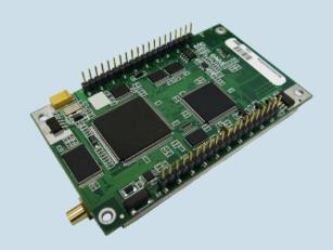
The MHX2420 features robust, low latency, secure data communications. It has full serial port and separate diagnostics port for real-time diagnostics without interrupting data communications. Excellent noise figure, superior interference rejection, very agile frequency synthesis, digital modulation, and matched filter detection, are among the many advantages to using the MHX2420.
