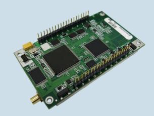
The MHX920A features robust, low latency, secure data communications. It has full serial port and separate diagnostics port for real-time diagnostics without interrupting data communications. Excellent noise figure, superior interference rejection, very agile frequency synthesis, digital modulation, and matched filter detection, are among the many advantages to using the MHX920A.
